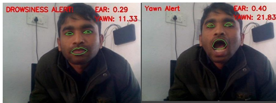
Figure 7: When a driver closes the eye to sleep Figure 8: Yawn alert when mouth opens
